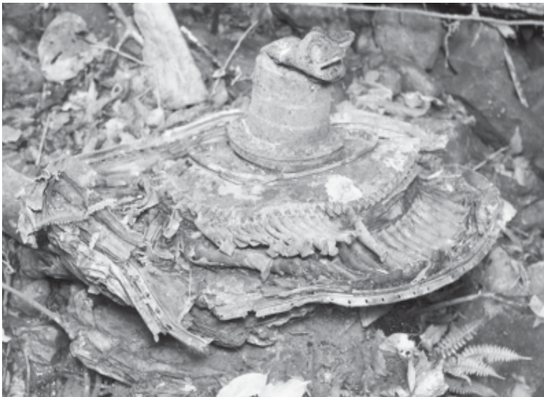
Wreckage of A84-231 engine found below the main crash site during Operation Magpie's Return. RAAF Official Image 8526964 014. Photo provided by the author.
