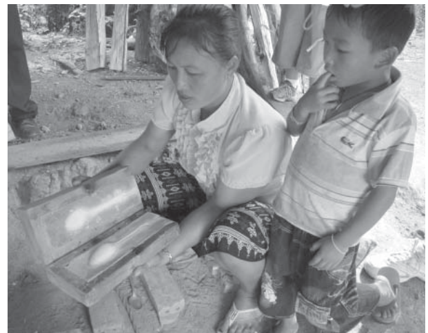
Above, feedstock for spoon foundry. Below, at backyard foundry woman displays a mold used to make aluminum spoons. Foundry operates when they need some money. Scrap aluminum is sold by local scavengers.
