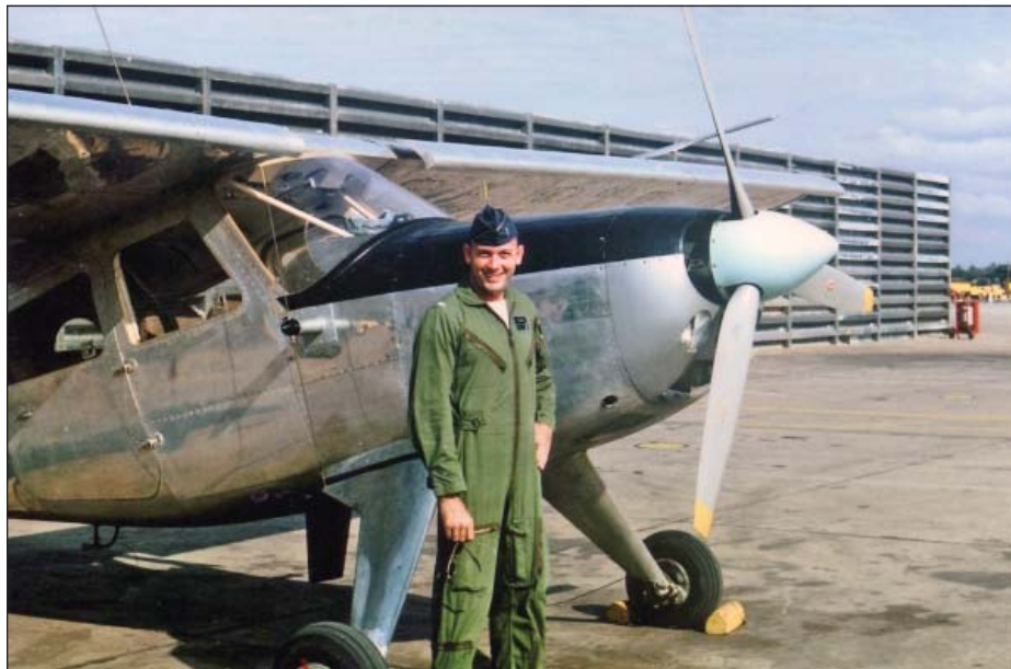
The author at Udorn RTAB to pick up passengers. Note the full-span wingslats. This feature was central to the U-10's remarkable STOL performance. Photos furnished by the author.
