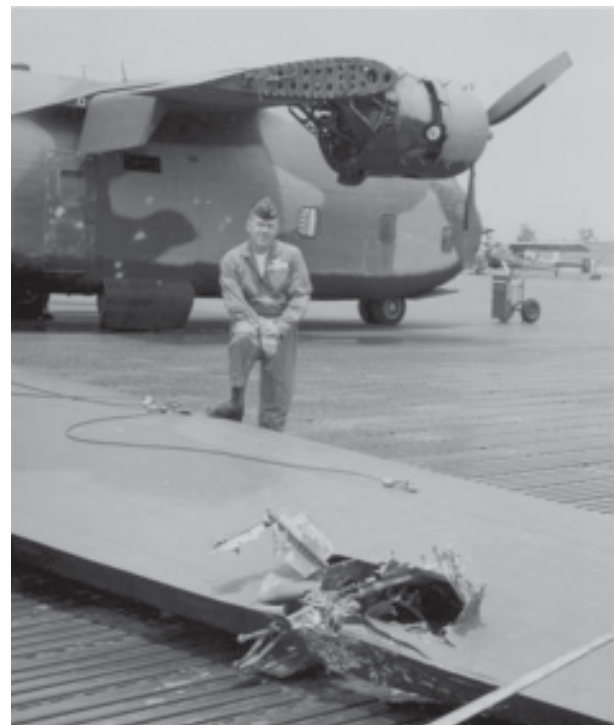
Warren Mewborn looks at 37mm shell damage to C-123 wing panel after a Route 912 mission. Photo from Mewborn.
