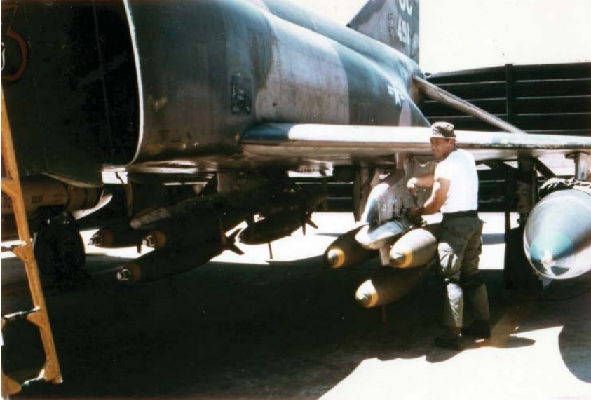
Finishing up a bomb loading operation on an F4-D at Udorn RTAFB, Thailand.
