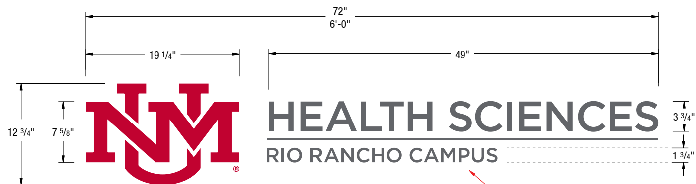
A ELEVATION - LOGO SHOWN AT 6' WIDTH SCALE: 1"=1'
