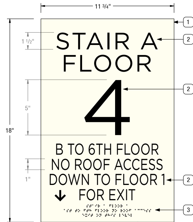
B SIGN FACE ELEVATION SCALE: 1:5 Braille is entire content of sign Example for this instance: stair A floor 4 B to 6th floor no roof access exit on this level
