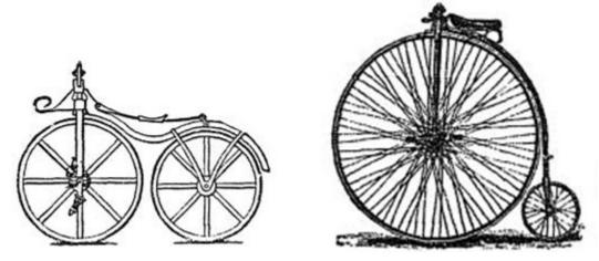
Since these were single speed fixed gear bikes, the front wheel had to be sized to allow both reasonable speed on the flats as well as the ability to accelerate and climb hills. Although standing
