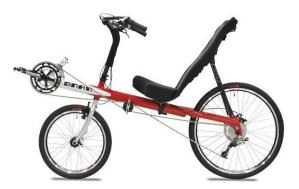
Proprietary G4 Bikes "Better Bikes for More People" • The Compact Long Wheel Base (CLWB) uses two large diameter wheels with pedals mounted high to clear the front wheel. The aerodynamic advantage of the pedals in line with the steeply reclined seat, along with the low rolling resistance of the large diameter wheels, makes this the fastest of the three configurations. It is also the hardest to ride.
