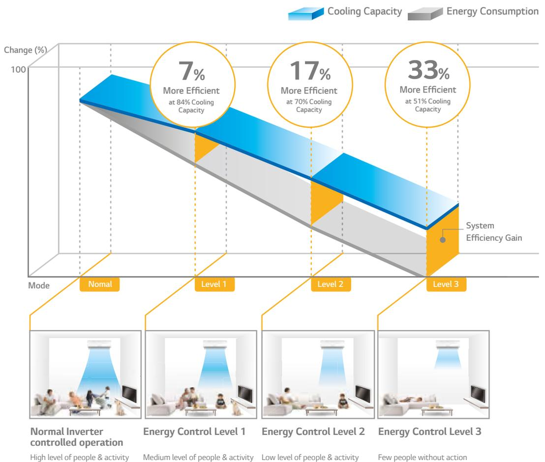
[Test condition] Test Standard AS/NZS 3823.1.1 / Normal Temperature (Indoor Temperature : 27°C, Outdoor Temperature : 35°C)
