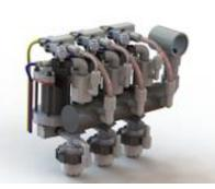
you get the same precision and accuracy if you are dispensing from 55 gal drums at 100 lpm or from bottles at 5 lpm. All metering parameters, including pumping speed, metering ramp-down, and metering valve frequency are under program control
