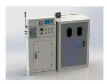
**MATECH** – Advanced transport phenomena of etched Bi-products results in a cleaner and sometimes particle reducing process. Also the single wafer linear scan technology allows for any size and shape of wafer or substrate. The linear scan gives single sided processing, while protecting the back side of the wafer.
