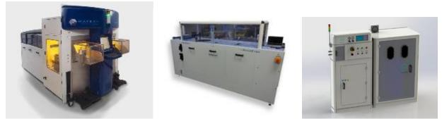
**MATECH** – Advanced transport phenomena of etched Bi-products results in a cleaner and sometimes particle reducing process. Also the single wafer linear scan technology allows for any size and shape of wafer or substrate. The linear scan gives single sided processing, while protecting the back side of the wafer.
