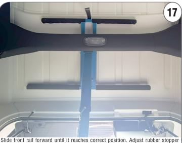
Slide front rail forward until it reaches correct position. Adjust rubber stopper screws so that top support bars touch the roof with rubber stoppers evenly supporting the top.
