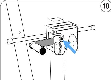
Remove nut from Hand Crank and install crank handle and nut to gear winch if necessary.
