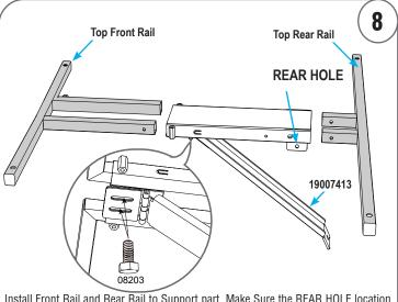
Install Front Rail and Rear Rail to Support part. Make Sure the REAR HOLE location first and install rear rail. Install bracket bar to top support with Bolt #08203.
