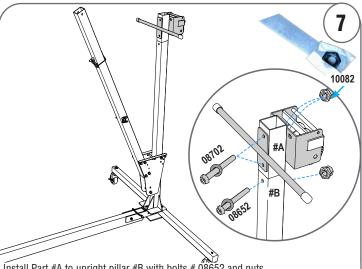
Install Part #A to upright pillar #B with bolts # 08652 and nuts.
