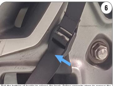
Pull the bottom of buckle to release the hook. Follow opposite steps to remove the EZ table from tire.
