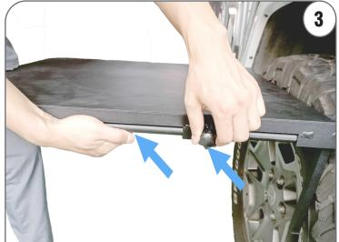
Diagram (3) Place table over tire. Hold table in place with pressure and hand pull the support bar towards you to make a secure tight fit. Then tighten the thumb bolt on each side of table.
