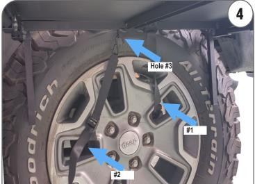
Diagram (4) Take hook side of webbing and feed through Hole #1 & #2 hooking onto Hole #3. Then adjust webbing tight with fasten to secure tightly to the vehicle tire
