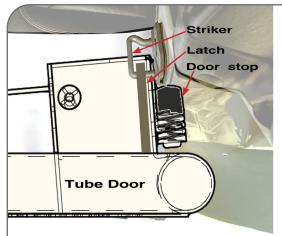
**CAUTION!** To avoid risk of injury latch mechanism must be properly adjusted before use. Inspect and adjust as necessary should wear alter alignment of latch and striker. Do not use door/latch if damaged.
