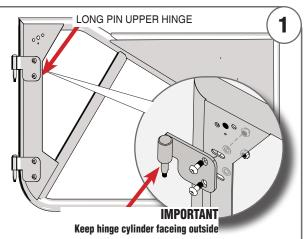
Attach the 2 door hinges to the new door using the 4 supplied M8x20 bolts and hardware. Leave the bolts snug only at this time, **IMPORTANT** Install the longer pin hinge on upper position of door and shorter pin hinge on lower position. The upper hinge with longer pin ,which can be use to assist in guiding the door into place.
