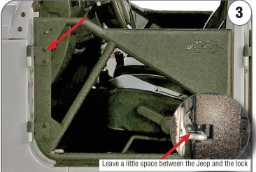
With the door closed, loosen the four screws from the hinges (using a #5 allen wrench and #13 open wrench), adjust door 2 directions position as needed and proceed to tightened the screws.
