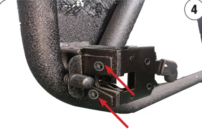
Adjust the rubber stop so the doors do not move when driving. Turn the rubber to adjust. Adjust the 2 screws if needed.
