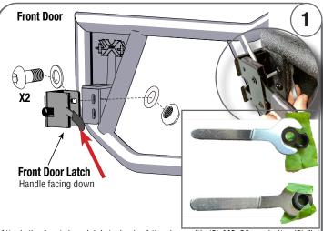
Attach the front door latch to back of the door with (2) M8x20mm bolts, (2) flat washer and (2) lock nut.DO NOT FULLY TIGHTEN hardware. Tap washer and nut on wrench to easy access back of door looking bracket.
