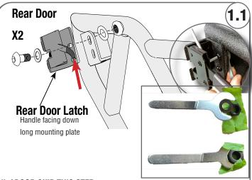
JL 2D00R SKIP THIS STEP. Attach the rear door latch to back of the door with (2) M8x20mm bolts, (2) flat washer and (2) lock nut.D0 NOT FULLY TIGHTEN hardware. Tap washer and nut on wrench to easy access back of door looking bracket.
