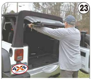
Pull the side bars in a little to go past the top edge of the window corner if needed.
