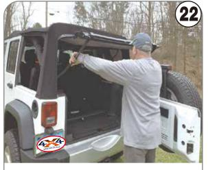
Lift the middle of the side bars up to fold the window down
