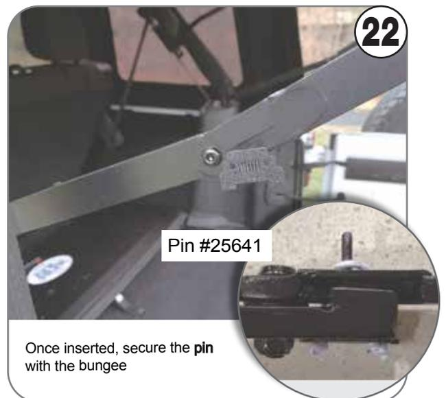
Once inserted, secure the pin with the bungee
