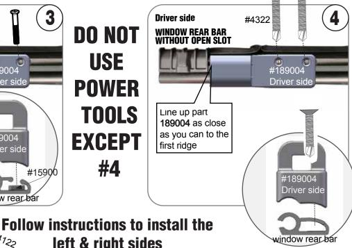
left & right sides 1. Remove rear window from Jeep 2. Use self-drill screw to make a hole 1/2" from the side 1/2" [12mm] 3. Drill a hole on each side of the rear window
