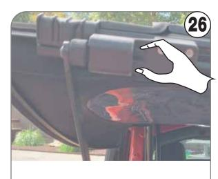
Press the ends to release the Support bar.
