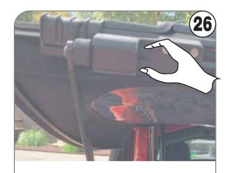
Press the end to release the support bar then roll back and secure with velcro strap
