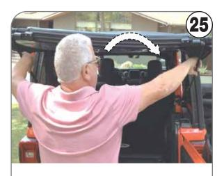
Bend the side bars up to fold the window down
