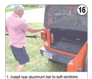
Use a wrench to adjust the tension if the bar does not drop down on its own.
