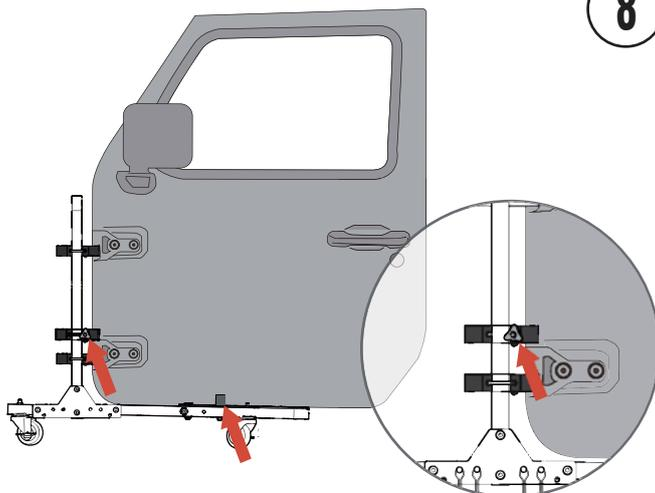
Slide down the safety hinge lock and thumb turn to tighten. This locks the doors in place for moving and storage.
