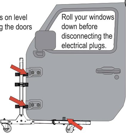
Place the doors on the cart with the bumpers on the outside and adjust the brackets so they are hitting the top of the door hinge brackets. Tighten the cart hinge brackets so they do not move. Make sure the cart is on level ground when loading the doors.
