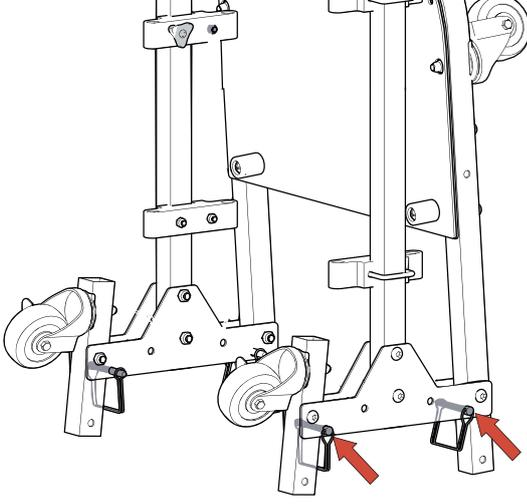
Place the pins in the bottom locking holes and store the other pins in the holes.
