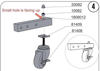
Place the bottom wheel Castor plate on wheel assembly to straight base tube. The small hole is facing up. Tighten the bolts and then place plastic caps on the wheel nuts.
