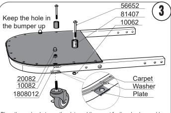
Place the washer between the plate and the carpet for the wheel assembly. Put the nuts on but don't tighten.
