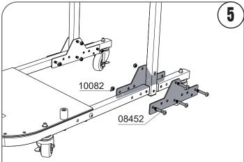
Connect the two plates and tubes together. Tighten the two middle upright tube screws. The folding outside screws should be snug not tight, so the bottom folding base swings up easily. The base should not drop down unless you pull it down.
