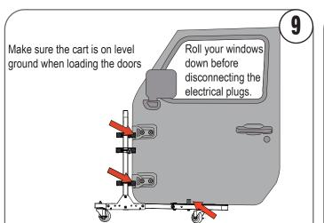
Place the doors on the cart with the bumpers on the outside and adjust the brackets so they are hitting the top of the door hinge brackets.
