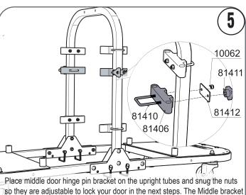
is a locking mechanism. This protects the doors from falling off when moving
