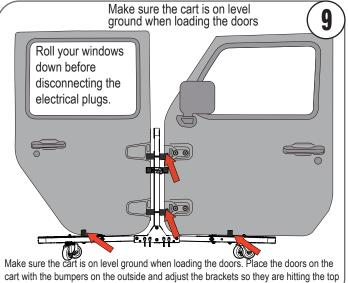
of the door hinge brackets. Tighten the cart hinge brackets so they do not move
