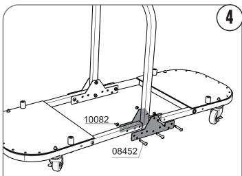
Connect the two plates and tubes together. Tighten the two middle upright tube screws. The folding outside screws should be snug not tight, so the bottom folding base swings up easily. The base should not drop down unless you pull it down.
