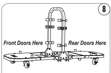
Roll your windows down before disconnecting the electrical plugs. Place the rear door from one side of the vehicle on the EZ-Door Holder Cart first. Then put the same side front door on EZ-Door Holder Cart. SLIDE THE MIDDLE LOCK IN THE DOWN POSITION when moving the cart to the other side. Take the doors from the other side off the same way. This distributes the weight on the cart.
