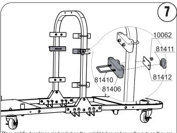
Place middle door hinge pin bracket on the upright tubes and snug the nuts so they are adjustable to lock your door in the next steps. The Middle bracket is a locking mechanism. This protects the doors from falling off when moving the cart.
