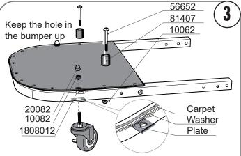
Place the washer between the plate and the carpet for the wheel assembly. Put the nuts on but don't tighten.
