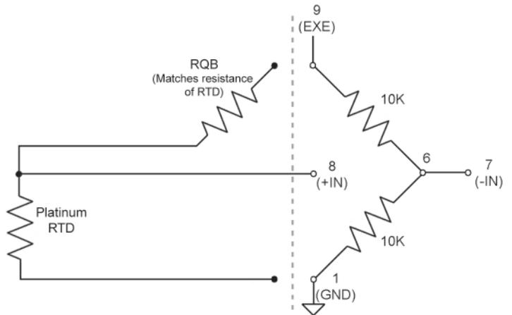
**NOTE:** For Platimun RTD configurations, the input dividers are set to OFF
