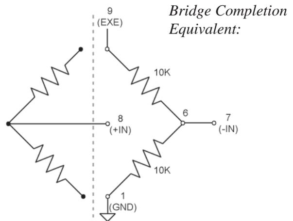
**NOTE:** For Half Bridge configurations, the input dividers are set to OFF
