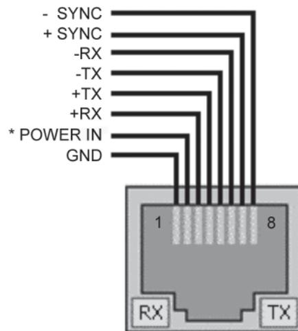
The POWER IN pin is internally configured at the factory for +5V, +12V or 0V. A label on the side nearest the COMM connector displays the POWER IN configuration.
