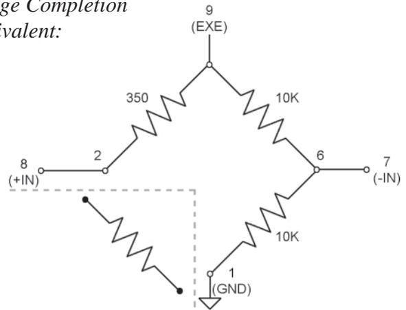
**NOTE:** For Quarter Bridge configurations, the input dividers are set to OFF
