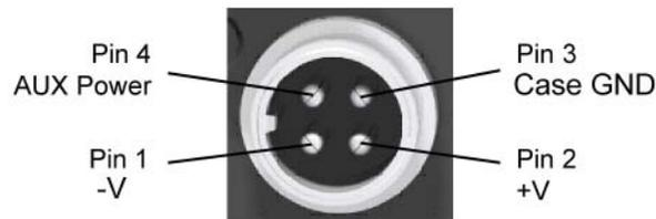
**WARNING:** When using a power adapter with a Titan device, always connect the adapter to the device before applying power. Never hot plug a device under any circumstances - hot plugging may damage the device!
