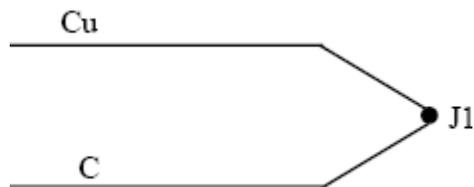
**Figure 1. Thermocouple Junction**
