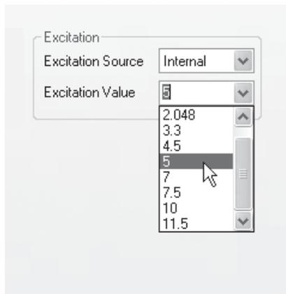
**NOTE:** When the Excitation Source is set to ‘Internal’, the excitation voltage is sourced from the Titan hardware. When the Excitation Source is set to ‘External’, excitation **must** applied to the sensor from an external source. Whenever external excitation is applied, the Excitation Value should be set to match this voltage.
