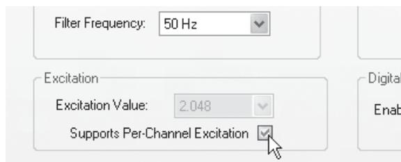
2. On the *Sensors* page, select the desired sensor type (a ‘Voltage’ sensor type is used for this example). Set the excitation source to ‘Internal’ and select the desired Excitation Value from the drop-down menu.
