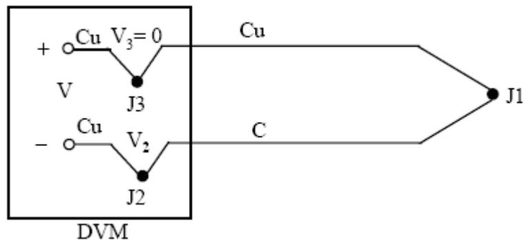
**Figure 2. Thermocouple attached to a Digital Volt Meter**
