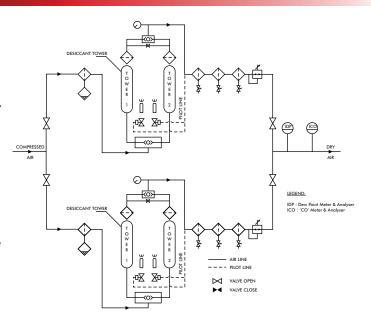
stand by dryer. So there is no need to stop the air dryers for maintenance. Purge saving system saves purge air upto 60% for a typical hospital load of 30% to 40%. Dewpoint and CO monitor enables to monitor dewpoint and CO levels as mandated by NFPA 99.
