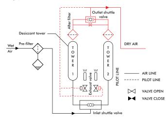
Regeneration Cycle: During this cycle, the sudden depressurization brings out water molecules trapped in the desiccant pores to the surface of the beads. A small portion of the dry compressed air from the
