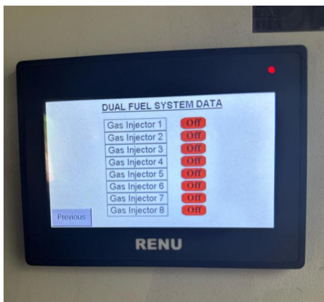
Real Time Input on Gas Injection Operation. Per Injector Functioning can be monitored.
