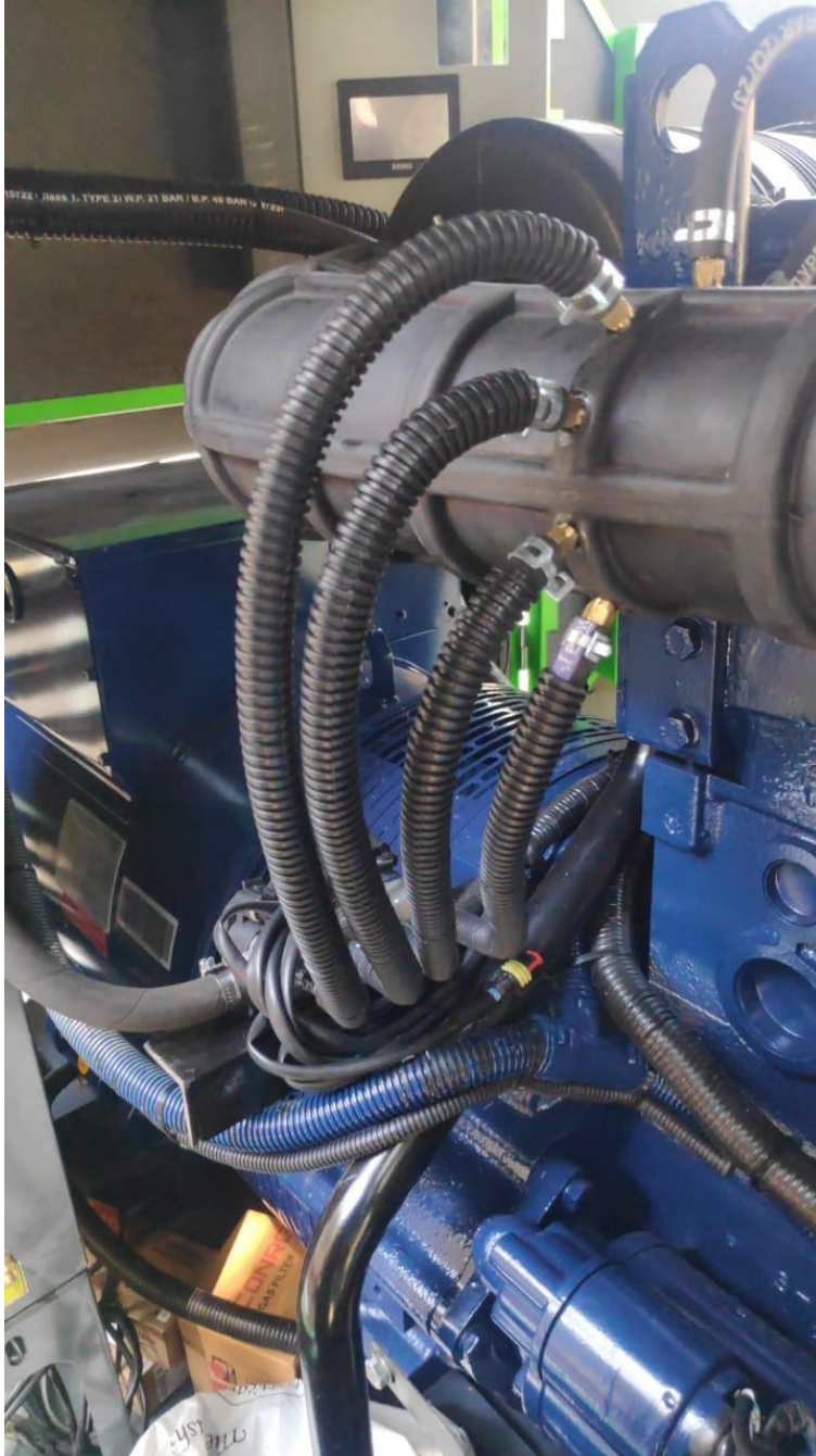
Injection Hose before Turbo for precise fuel injection as per Engine Capacity.
