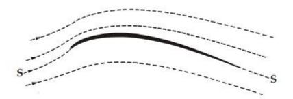
Airfoil Shape - Force generation is same as board except with a curved shape for better efficiency in producing driving force from airflow.
