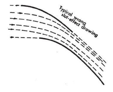
If this were the case, instead of the main billowing out when "backwinding", the higher speed of airflow through the slot would create low pressure in the slot and cause the luff of the main and jib to be pulled towards each other.
