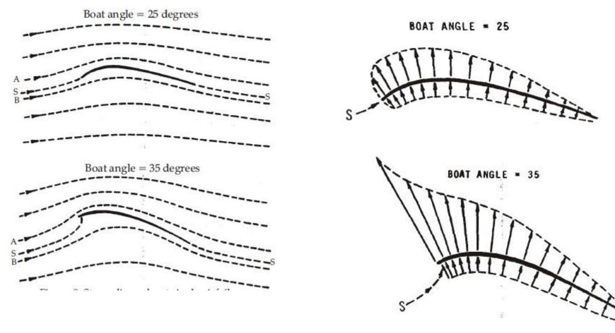
Greater chance of separation from the sail at a higher angle of attack due to deceleration of airflow.
