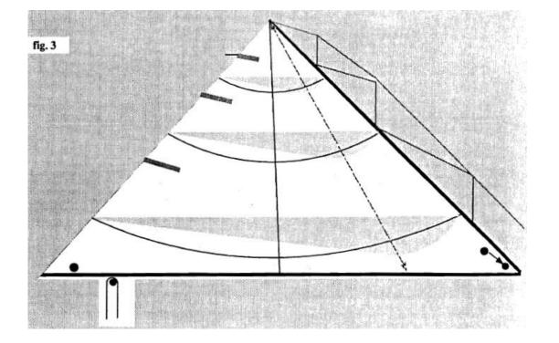
Steering Angle – The ability to deviate from the course sailed and still have the sails working properly and not stalling. The position where the draft is deepest should be at 45%-50% aft of the mast to give the best sail performance.
