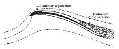
**Separation**- When the increase in pressure due to air slowing down is too great, the airflow separates from the surface of the sail. This may be caused by overtrimming the sail, hooking the leech, or having too much camber in the sail.
