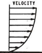
Fluid Viscosity: The force needed to slide the sheets of paper over each other.
