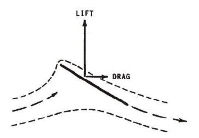
Force diagram shows that a force called 'lift' that is perpendicular in direction to the air flow is generated due to the pressure difference from air flow over the board.
