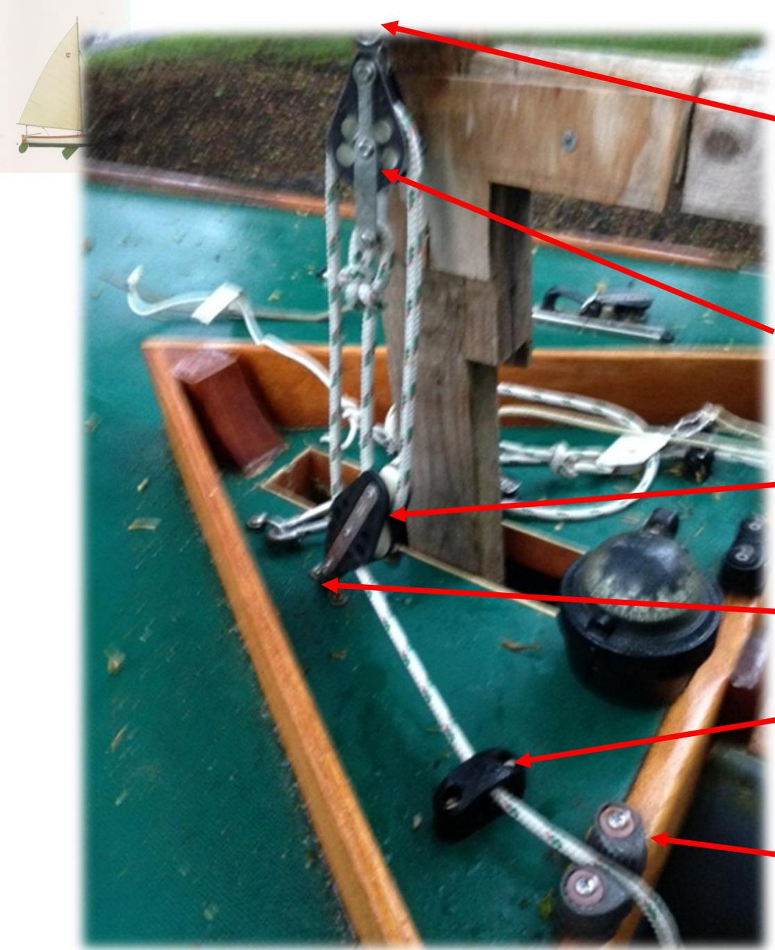
Brummel Hooks attach Jib Halyard to Tackle with tail of Halyard coiled below deck
