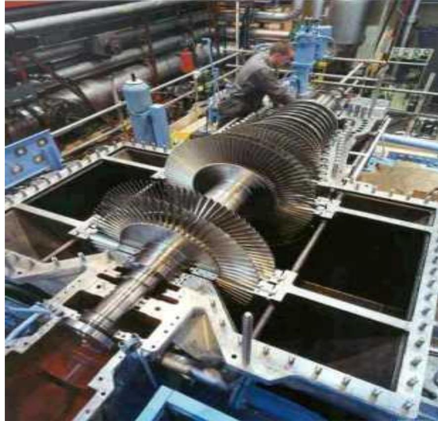
Rotor of 8 MW Steam Cogeneration Unit
