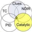
= Cat bead is the only direct reading of flammability
