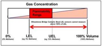
While the catalytic bead sensor is the most common LEL sensor in handheld detectors, alternative techniques need to be considered
