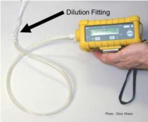
Some dilution fitting capable detectors automatically calculate the corrected reading accounting for the dilutant gas. This kind of capability is typically only found on high-end detectors.
