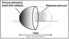
A coiled wire is used to maximize the surface area of catalyst. It is put into a porous ceramic bead to keep it from flexing like a "Slinky" and shorting out on itself. This adds to the durability of the sensor and helps it to resists shock.
