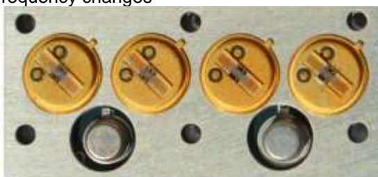
Array of 4 SAWs with 2 heaters
