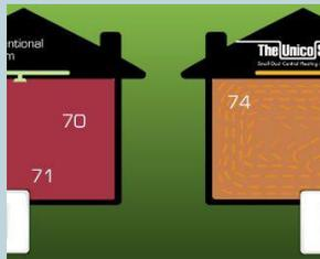
This illustration shows the Unico System with a slightly higher room temperature but even temperatures. Even temperature comparison
