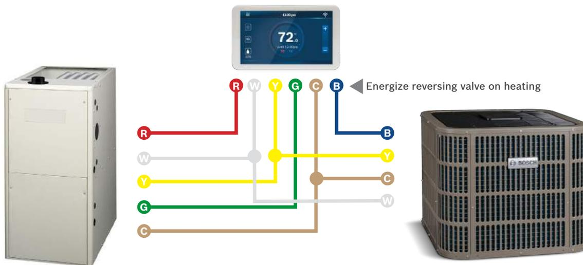
As you can see in Figures 1.1 & 1.2, only four 24V control wires are required for heat pump operation
