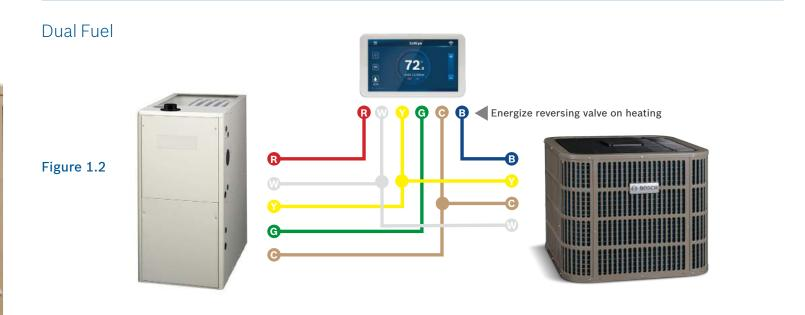
As you can see in Figures 1.1 & 1.2, only four 24V control wires are required for heat pump operation
