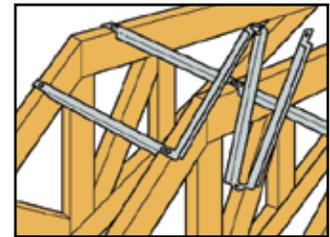
Example of a non-structural metal fold-out spacer.
