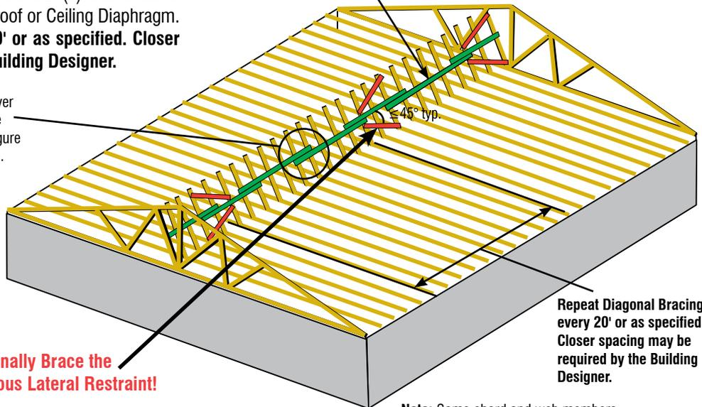
**Always Diagonally Brace the Permanent Continuous Lateral Restraint!**
