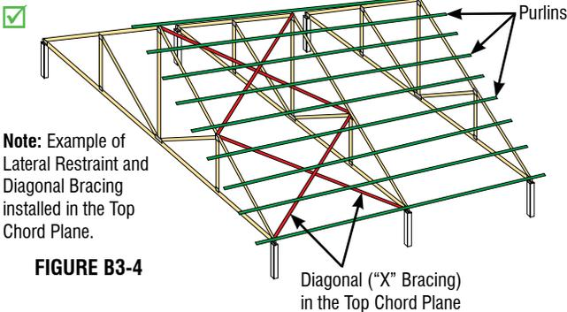
Note: Example of Lateral Restraint and Diagonal Bracing installed in the Top Chord Plane.
