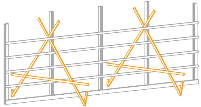
A-Frame Ground Bracing Perpendicular to the Wall
