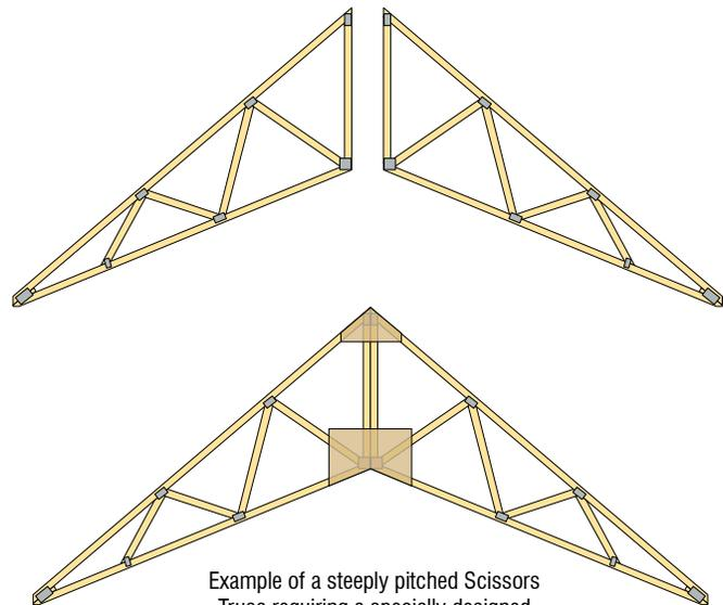
Example of a steeply pitched Scissors Truss requiring a specially designed field splice at the top and bottom peak. See TDD for splice details.
