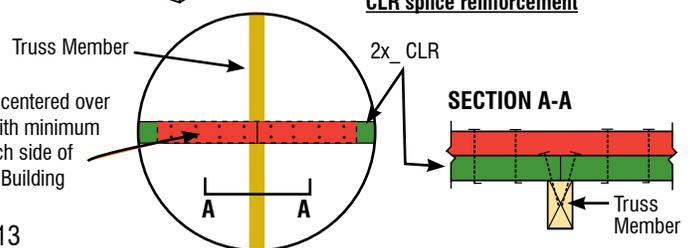
**\*\*IMPORTANT NOTE:** Install Bottom Chord **Temporary** Lateral Restraint (BCTLR) in rows no more than 15' on-center (o.c). Install Bottom Chord **Permanent** Lateral Restraint (BCPLR) at the spacings specified in the TDD and Construction Documents. The maximum on-center spacing of permanent Lateral Restraint is 10' but can be less if required by the TDD and/or Building Designer.
