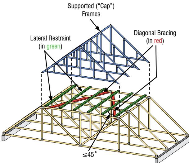
**Note:** Some Lateral Restraint and Diagonal Bracing not shown for clarity.
