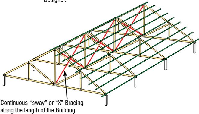
Continuous "sway" or "X" Bracing along the length of the Building
