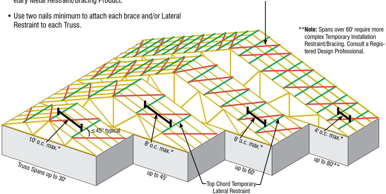
**\*NOTE:** Maximum spacing for Top Chord Temporary Lateral Restraint
