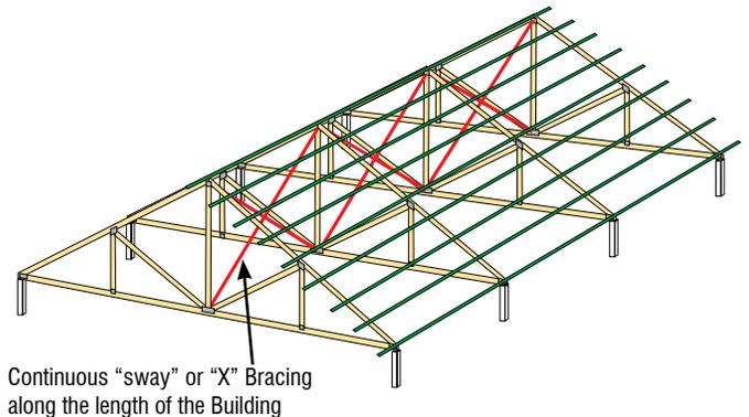
Continuous “sway” or “X” Bracing along the length of the Building
