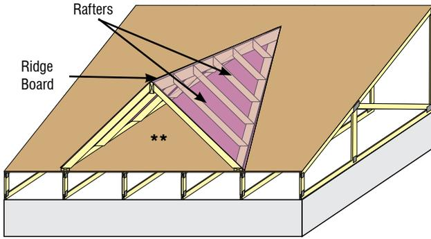
For conventionally framed dormers, as shown in this figure, the Top chords of the supporting Trusses beneath the dormer must be restrained and Braced with Structural Sheathing, as shown, or with rows of Lateral Restraint and Diagonal Bracing, to prevent buckling under Load. See NOTE below for assumed flow of Loads to Trusses depending on the method used to frame a valley.
