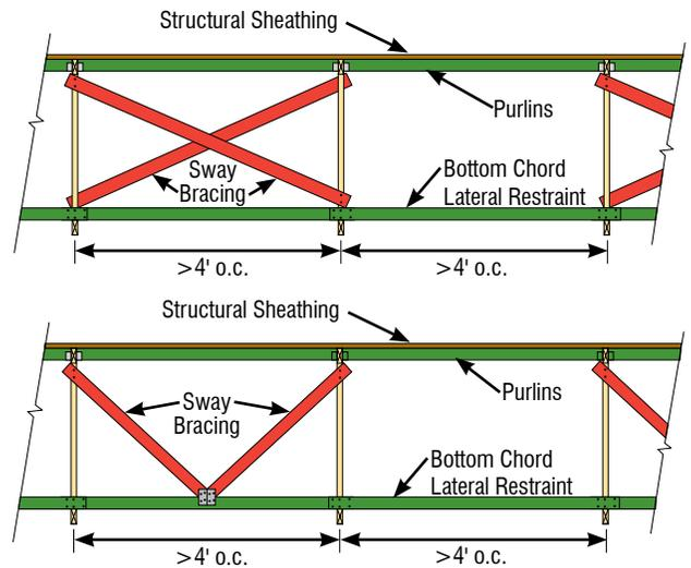
**Note:** Reinforce Lateral Restraints and Bracing, as required, for Truss Spacings greater than 4' o.c.
