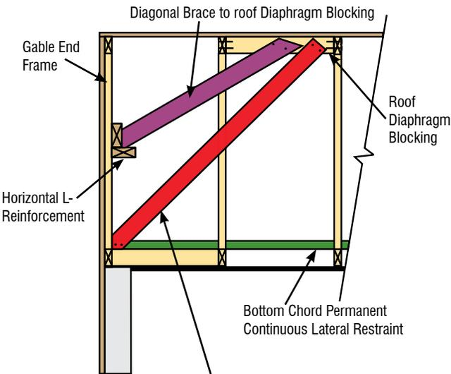
Gable end wall permanent Diagonal Bracing. Locate in line with Bottom Chord permanent CLR or as specified in the Construction Documents (see Figure B3-40, page 50).
