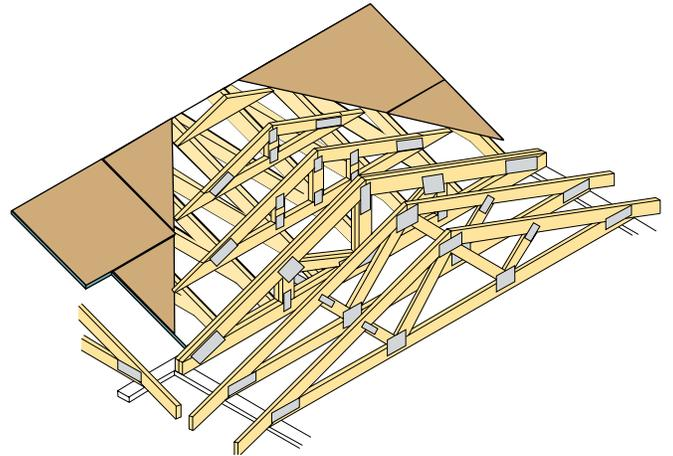
No Structural Sheathing attached to the Top Chords of the supporting Trusses beneath the Valley Set frames. The on-center spacing of the Valley Set frames, as measured along the slope of the Top Chord of the supporting Trusses, must be less than or equal to the maximum Purlin spacing specified on the TDD for the Top Chord of the supporting Trusses. Add Diagonal Bracing to the Top Chord Plane of the supporting Trusses if the Valley Set frames are ≥ 20' in length.
