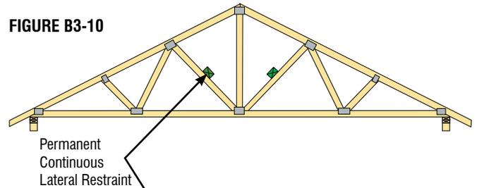
Lateral Restraint lapped over two Trusses or CLR splice reinforcement. Refer to Figure B3-7 for more information.
