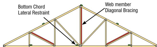
Apply Diagonal Bracing to Webs that are near each row of the Bottom Chord Lateral Restraint. See Figure B2-35 for spacing of Bottom Chord Lateral Restraint.
