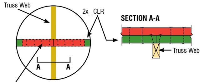
Minimum 2' 2x Scab block centered over Web/CLR splice. Attach to CLR with minimum 8-16d (0.135x3.5") nails each side of web/CLR splice or as specified by the Building Designer
