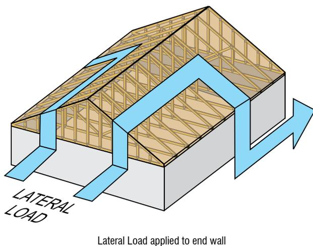
Lateral Load applied to end wall
