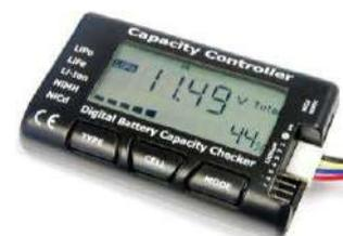
*Figure 23: Battery tester*
