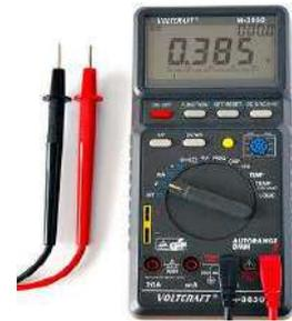
Figure 17: Digital Multimeter (Source: commons.wikipedia.org)
