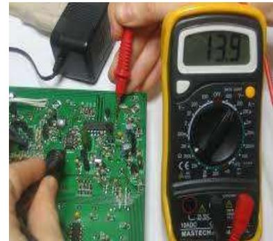
Figure 30: Using a Multimeter
