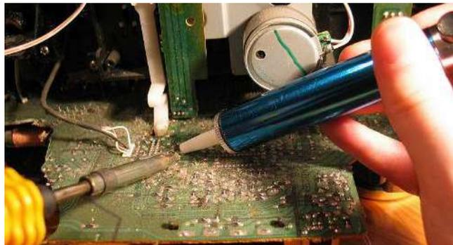
*Figure 28: Desoldering*
