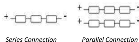
*Figure 36: Diagram Showing Series and Parallel Connections*
