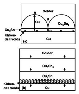
**Figure 4.** Schematics of how microstructure between solder and copper evolves from (a) as soldered to (b) prolonged exposure to high temperature. Reprinted from Ref. [16], with the permission of AIP Publishing.
