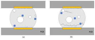
**Figure 2.** (a) Types of voids related to solder paste and alloy. (b) Relationship between macro voids and crack initiation/propagation.
