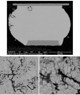
Figure 3. Example of shrinkage voids in Pb-free alloy.
