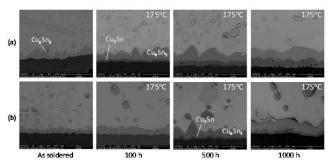
**Figure 5.** Evolution of IMC micro voids upon aging at 175°C for (a) Sn-4Ag-0.5Cu, and (b) Sn-0.3Ag-0.7Cu-X.
