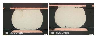
Figure 8. Effect of voids in mechanical reliability drop shock test.
