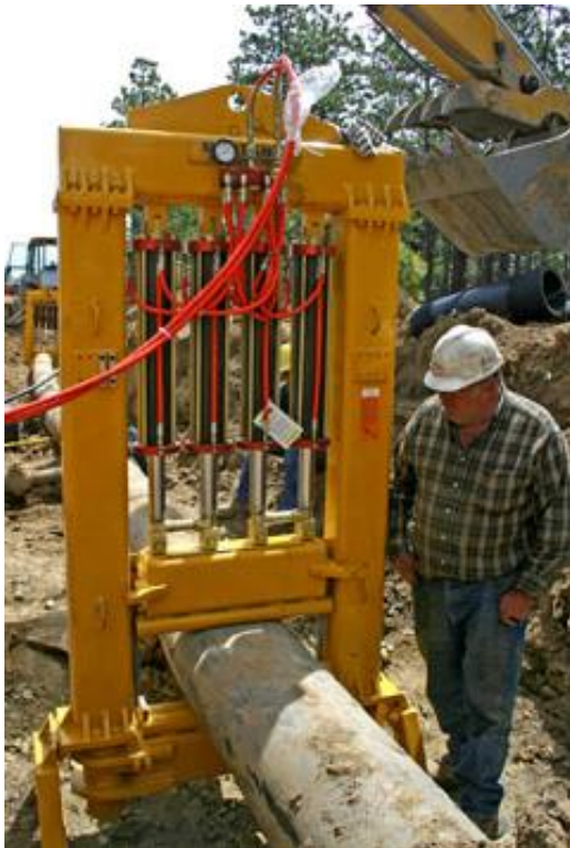
Figure 42. Traditional squeeze tool for 16" PE pipe
