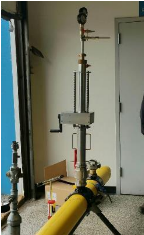
Figure 6. Kleiss BZA-4G1 stopping system attached to an electrofusion PE fitting and PE pipe
