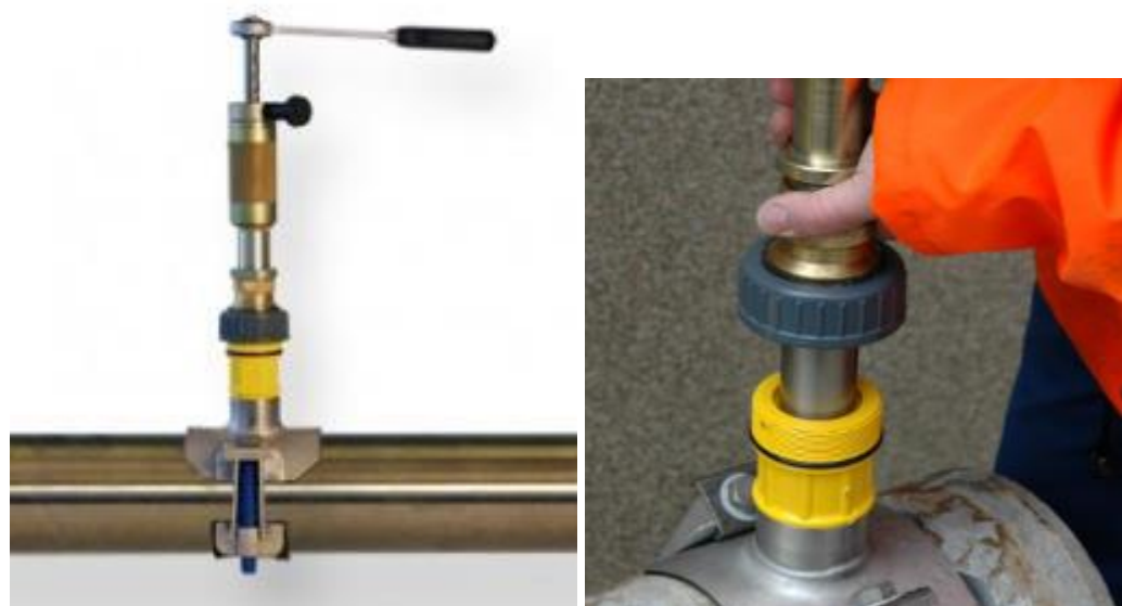
Figure 9. P3 (low pressure) hot tapping tool
