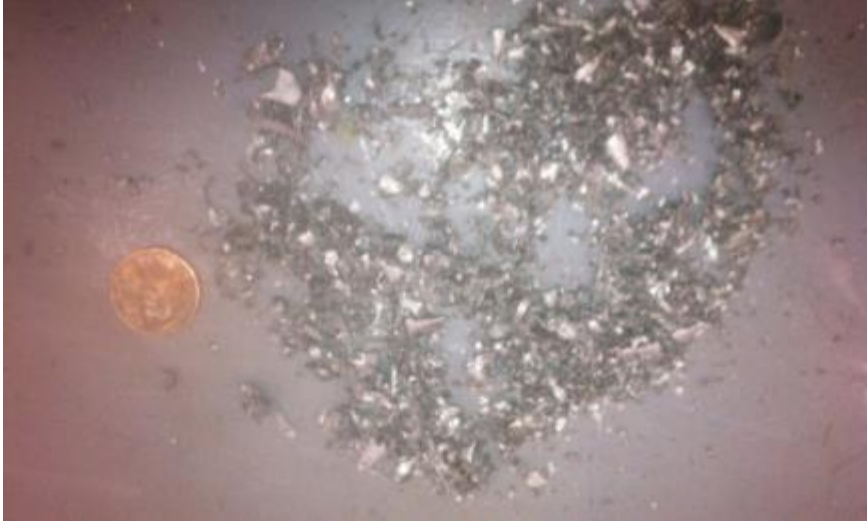
Figure 31. Steel shavings used for the debris test
