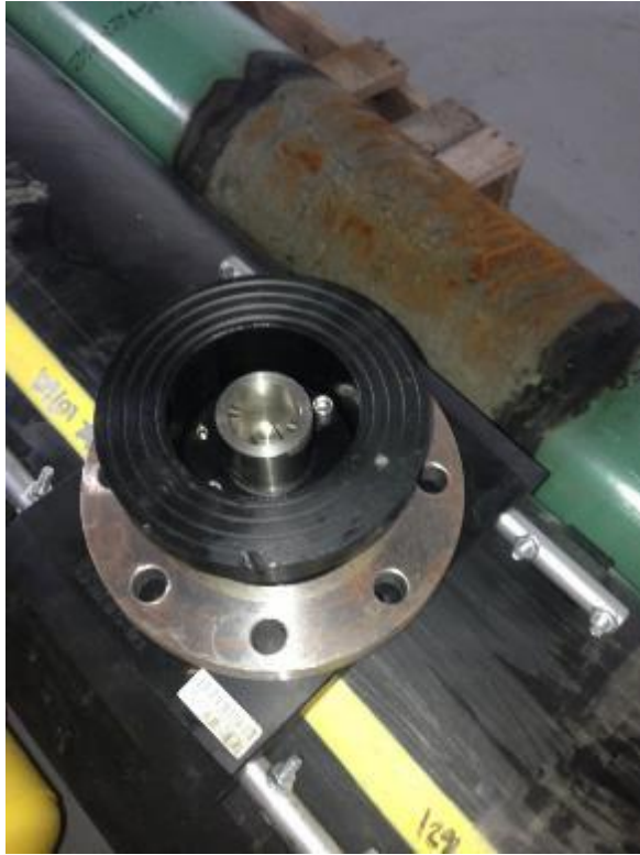
Figure 7. Kleiss electrofusion PE fitting and completion plug for 10” – 18” PE pipe
