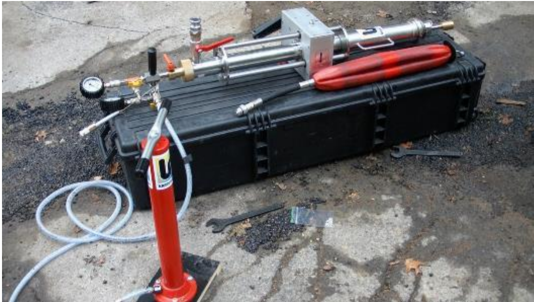
Figure 21. Kleiss BZA-4-G1 stopping system with carrying case and inflation pump
