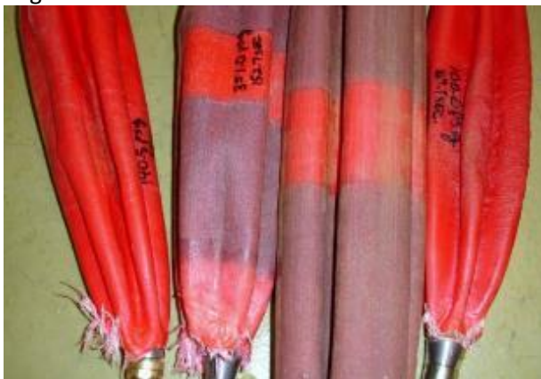
Figure 29. Kleiss stoppers with and without the grit coating (dark strips on surface of bag)
