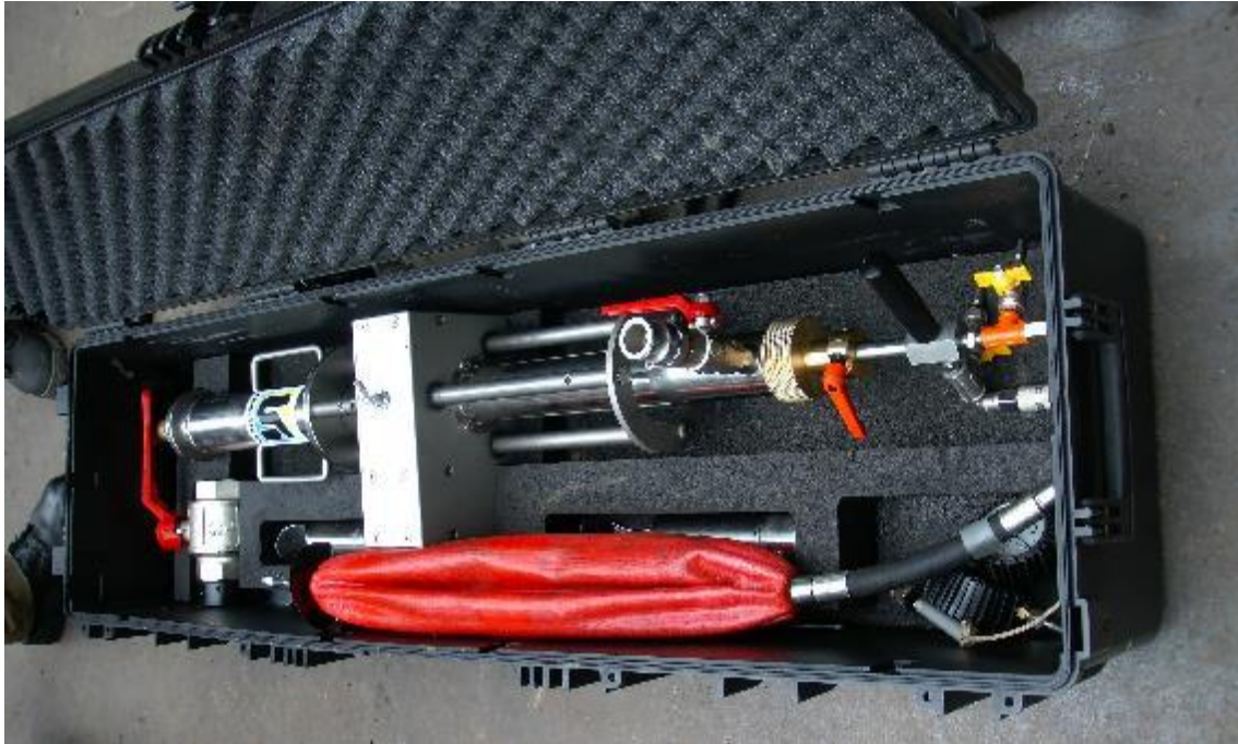
Figure 50. Kleiss BZA-4-G1 stopping equipment used to stop off the flow in the 8” steel pipe
