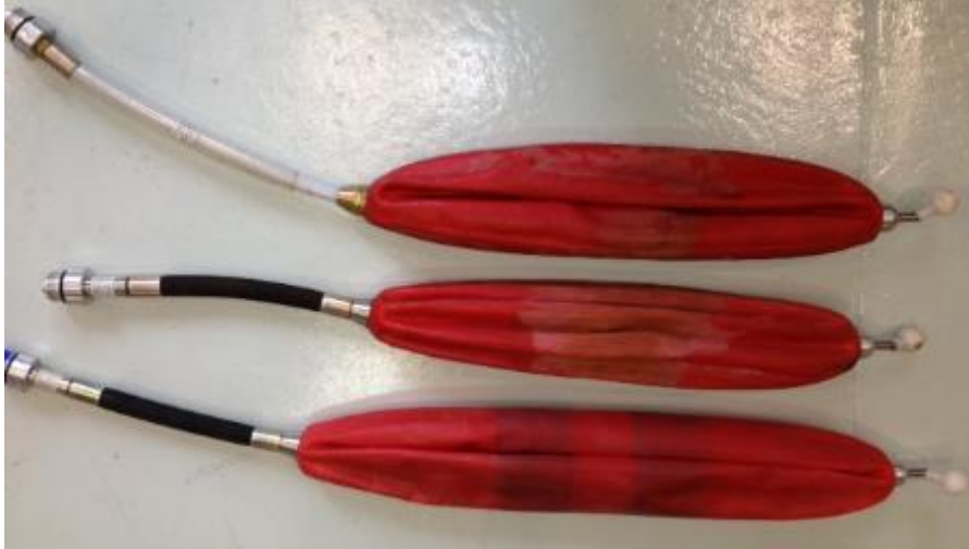
Figure 30. Kleiss medium pressure (15 psig) progression of bag design – top bag is the original with poly tube and no grit – middle bag was modified to include hydraulic hose and connector – bottom bag was modified to include hydraulic hose/connector, and grit on bag surface.
