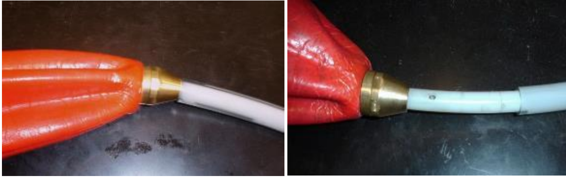
Figure 27. 15 psig stopper new (left) and 15 psig stopper after bag slid forward in pipe
