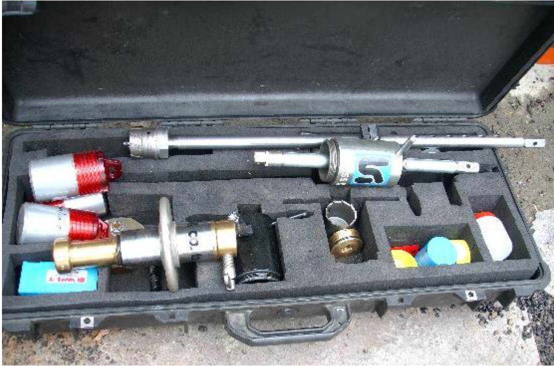
Figure 48. Kleiss tapping equipment used to tap the 8” steel pipe
