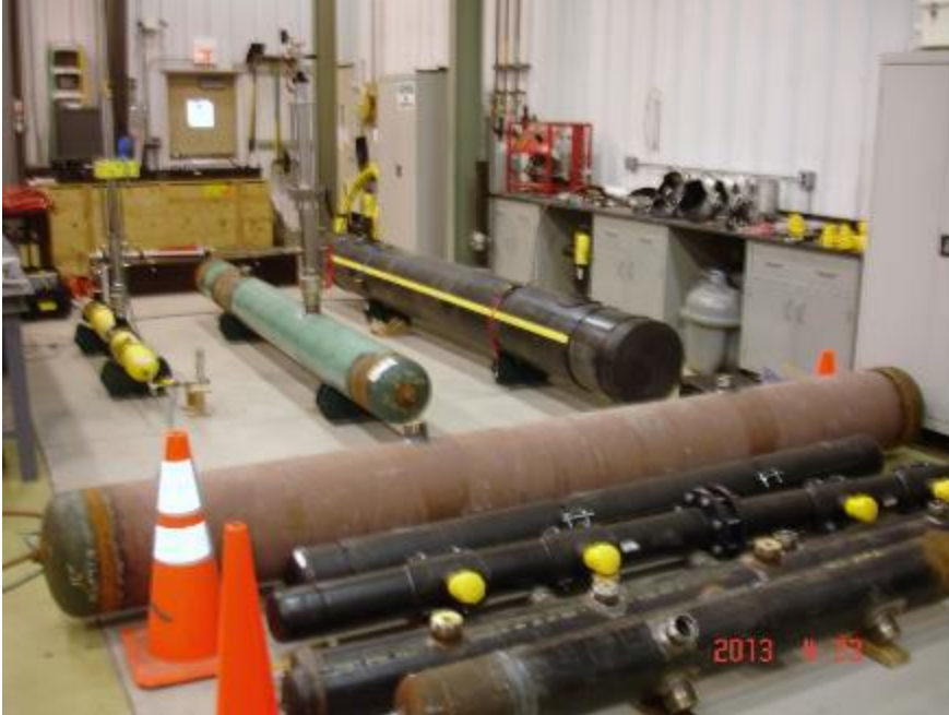
Figure 26. Cast iron, steel, and PE pipe to evaluate the Kleiss system
