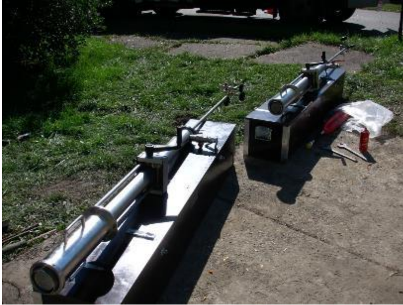
Figure 39. Kleiss BZA-1-G1 medium pressure stopper units used to stop off the flow in the 16” cast iron pipe
