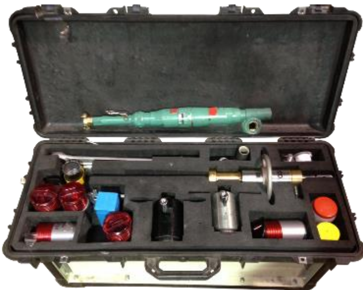
Figure 12. Hot tapping kit with all necessary accessories
