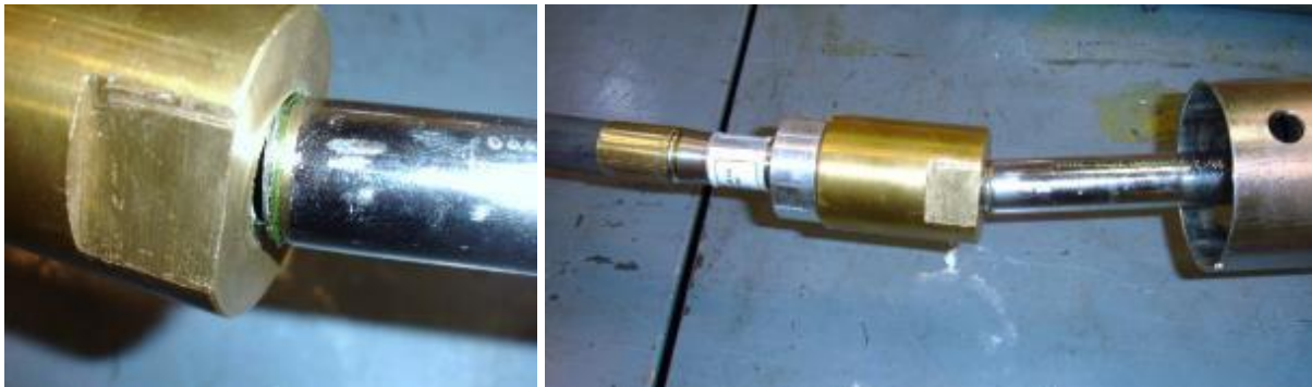
Figure 28. Stem of stopping machine cracked with newly designed 16” stopper at 15 psig pipe pressure
