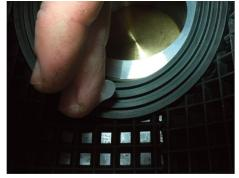
3. Apply a thin film of seal lubricant to the rubber ring gasket on the upper portion of the fitting. Do not over lubricate. (Use a lubricant such as Super Lube or similar synthetic grease.)
