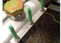
5. Install the spreader plates, washers, and nuts onto each bolt.
