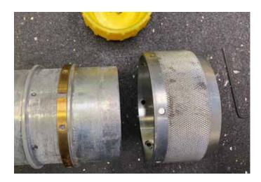
2. Remove the brass collars to clean the chute.
