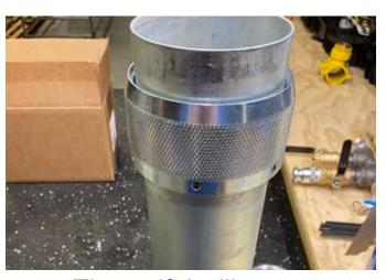
The swifel will move freely on the chute. Adjust screw tension for proper movement.
