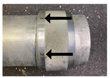
1. Remove the (6) set screws from the brass collar beneath the swifel.
