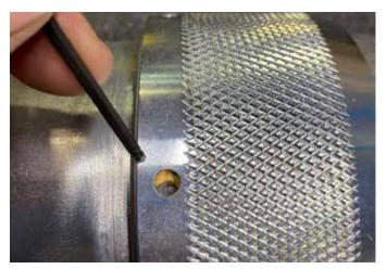
3. Replace brass collars and install new swifel. Use allen wrench to adjust alignment of the swifel and collars.
