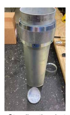
Standing the chute upright can aid in swifel installation and tension adjustments.
