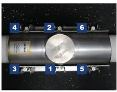
5. Follow the torque pattern detailed in the picture. Torque bolts gradually in passes.
