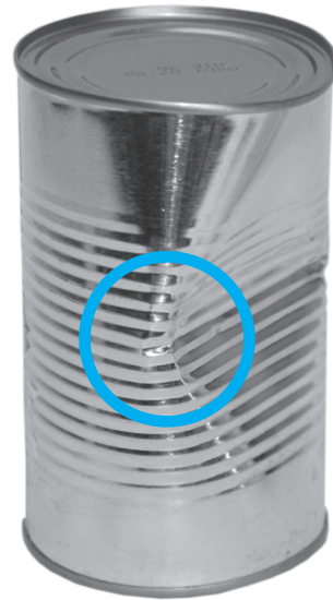
Sharp dent or dent on seam
