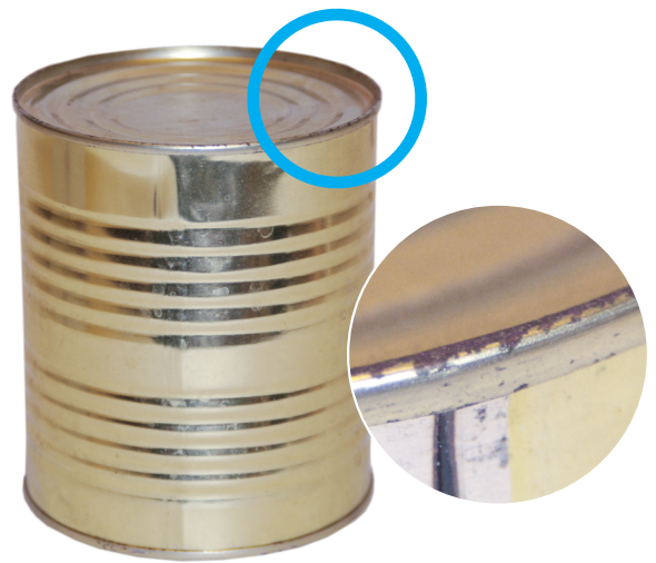
Pitted rust or leaking
