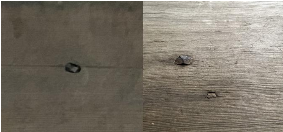
Figure 24: This photo shows two nearly identically wrought large nails, the left example was found on the back of a James Crow Shop piece in storage at MESDA, the right example is on the blue press. Note the small nail on the right example driven down through the top into the upper molding.
