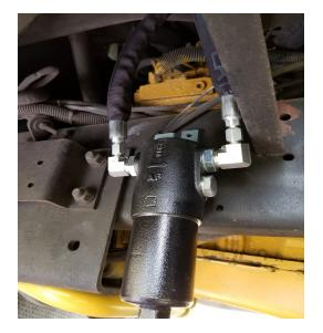
Frame mounting the filter unit provides many benefits for the end user. The bottom of the filter bowl is slightly higher than the oil pan and provides easy access similar to draining your engine oil.
