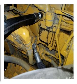
As you can see, NO modifications are required to any original components on your engine. At any point you could remove this kit, install the original steel tubing and move the IFS kit to another coach.
