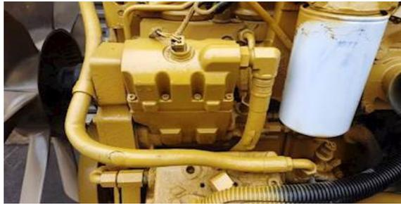
The photo below shows the connection points. Lower hose shown is the HEUI outlet and connects to the filter inlet. The top hose connects to the head port from the filter outlet.
