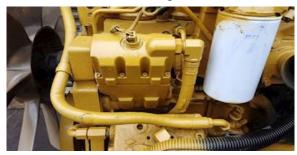
The photo below shows the connection points. Lower hose shown is the HEUI outlet and connects to the filter inlet. The top hose connects to the head port from the filter outlet.
