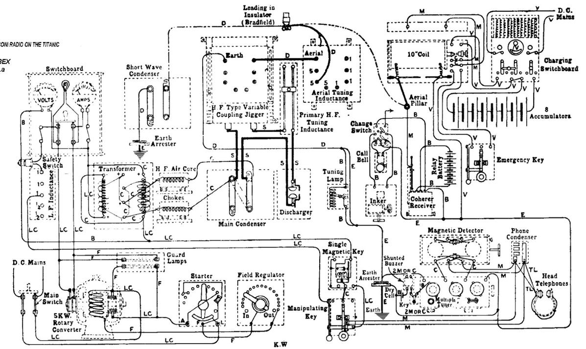
Reference to Wiring: LC =  $\frac{1}{2}$  Lead Covered. I =  $\frac{1}{2}$  Lead Covered. M = Silk Marconi Flex. C = No. 10 Bare Copper. B = Bell Wire.
