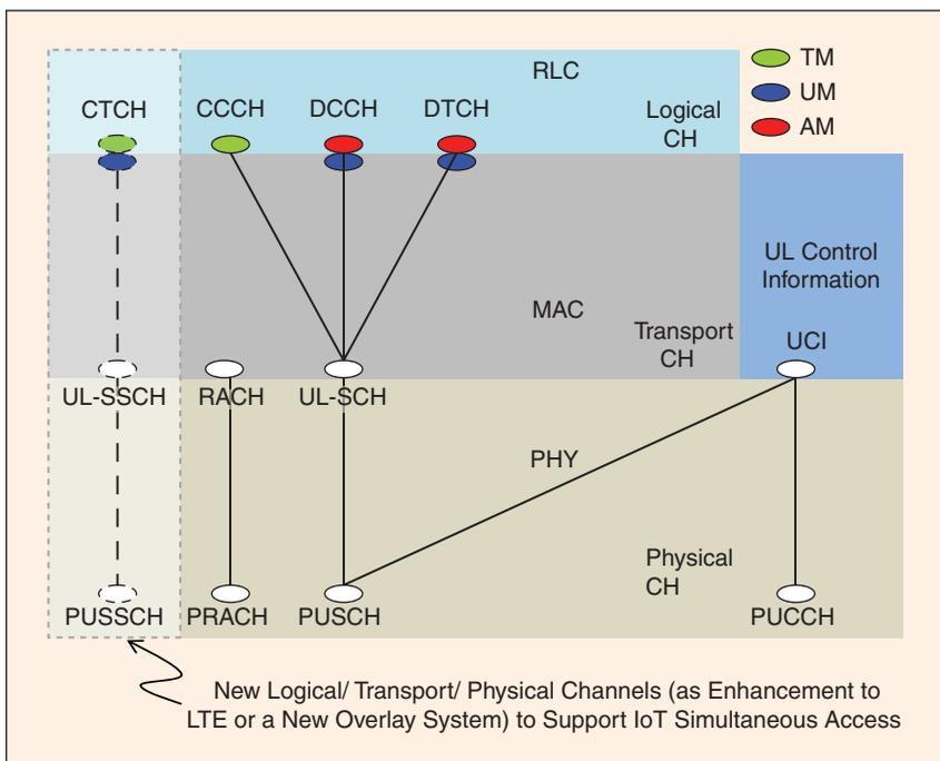
**FIGURE 6** UL channel mapping for the IoT air interface.
