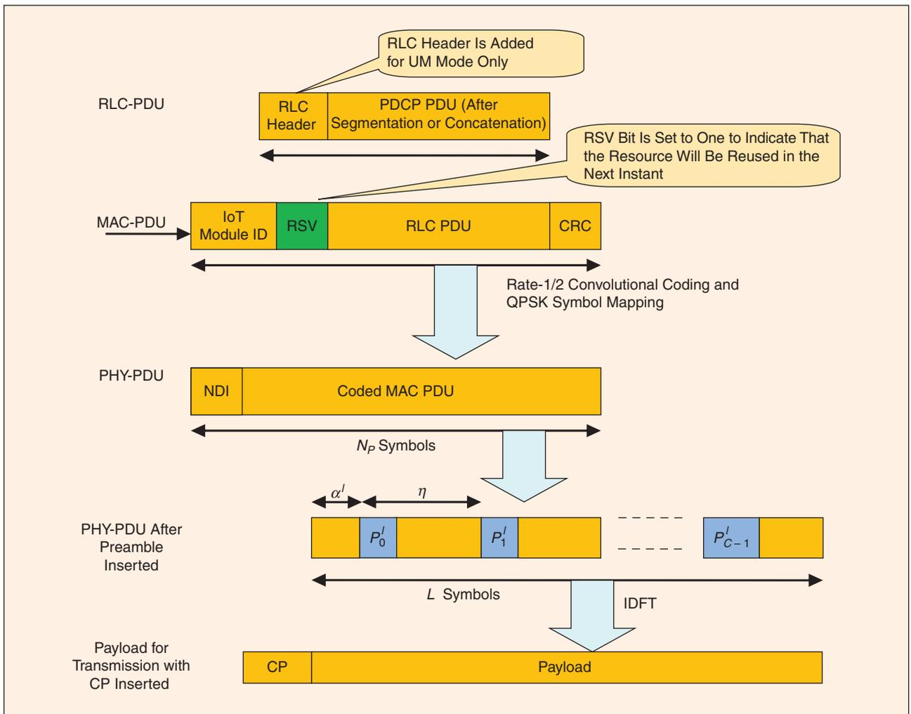
**FIGURE 7** The PUSCH payload transmission format.
