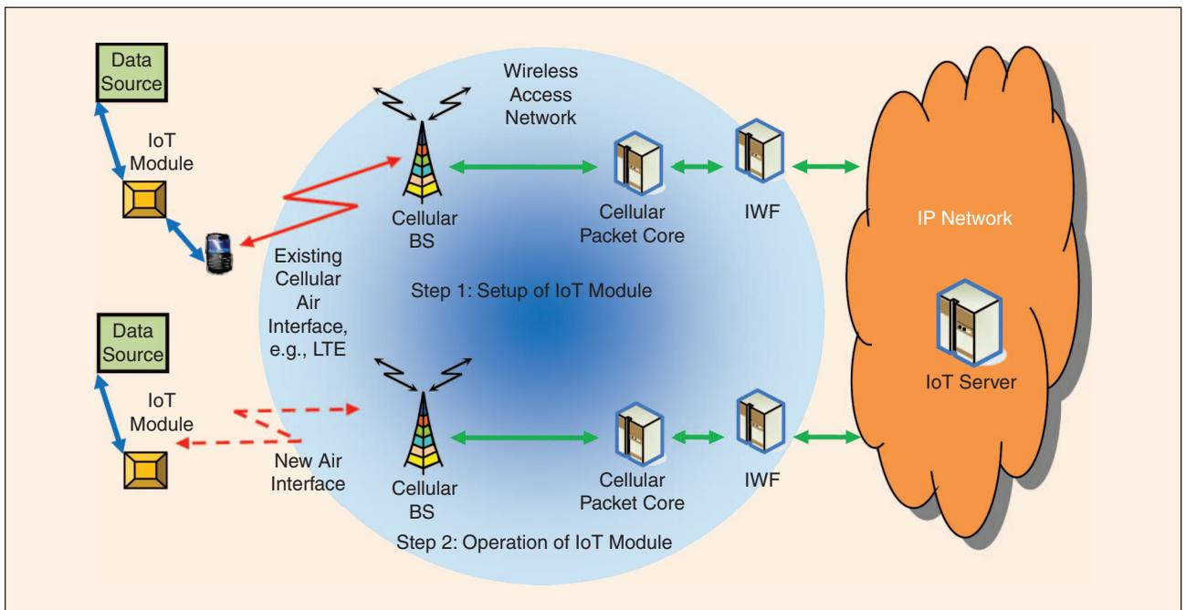
**FIGURE 2** The IoT wide-area communication system: initial setup and operation.
