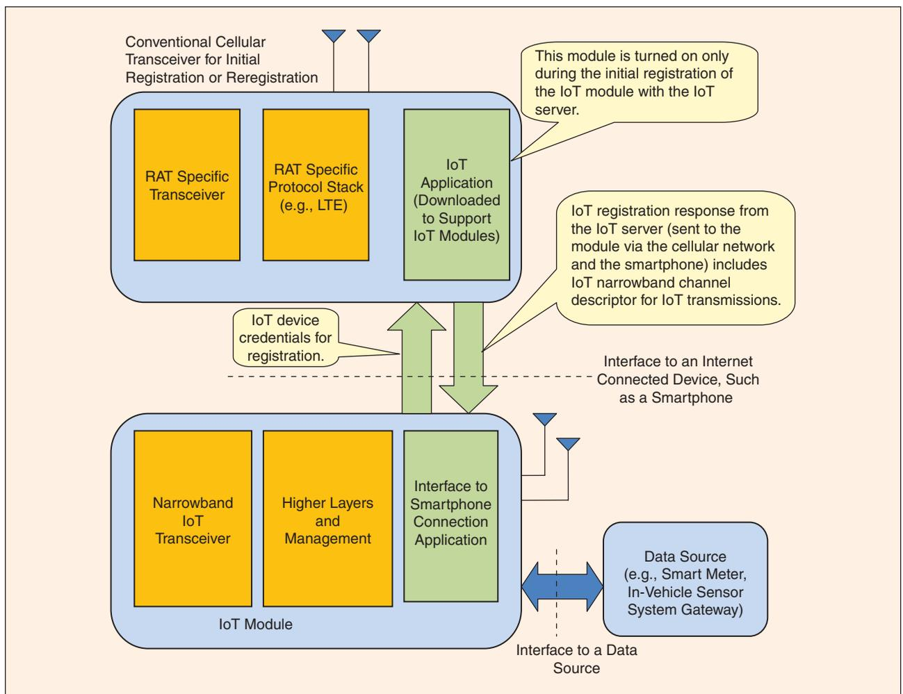
**FIGURE 1** The IoT module for the wide-area communication system.
