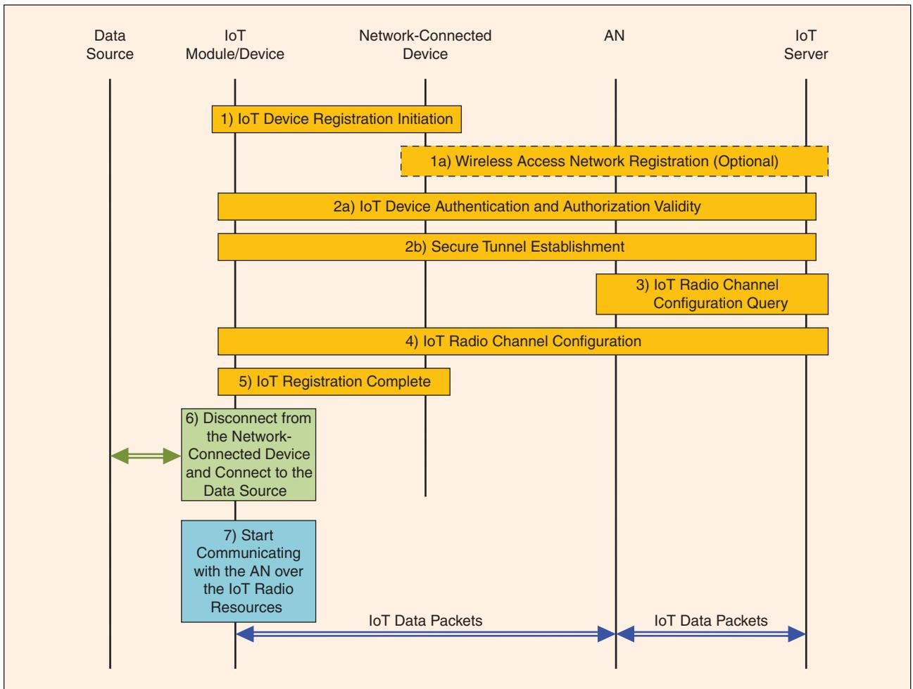
**FIGURE 3** The IoT module setup procedure.
