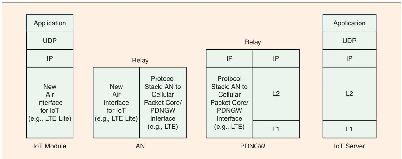
**FIGURE 4** The protocol stack for IoT air interface.
