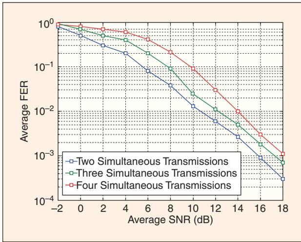
FIGURE 8 System UL FER performance.
