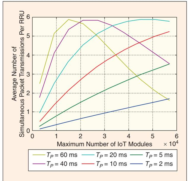
FIGURE 9 The performance of the simultaneous access contention mechanism.
